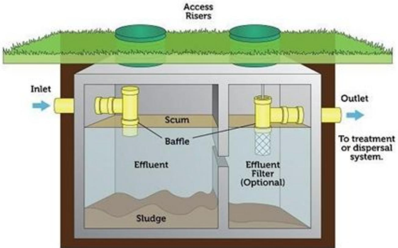
Figure 3: Septic tank schematic
