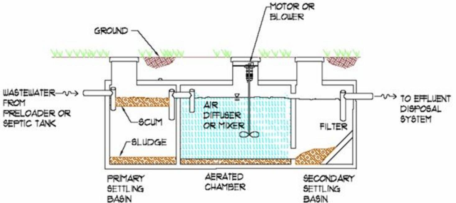
**Figure 4: Example Aerobic Treatment Unit (ATU) schematic**
